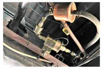
this: Measured Pressure on this Pulsating Pump is 6.5 psi. I'm certain my carbs can handle that much pressure but I will check all my connections once it is installed. Goes right back on the
