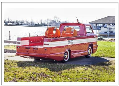
1961 Chevrolet Corvair Corphibian amphibious vehicle concept. Developed from a rear-engined Corvair Rampside pickup, it has a fiberglass hull and propellers driven hydraulically off the truck's engine. Throttle and rudder controls are located in the truck's cab and the bed.
