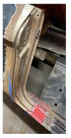
a donor car which had to be an early convert because he wanted the door to be built without that big square frame on the 4dr. The Convertible door's glass rises with no frame around it. This allows the glass to be
