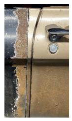
cut to the shape of the new top. Allowing Dave more design flexibility. The photo also shows nine more inches of shiny new floor. Cutting off the front of that side panel from the Convert and
