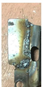
Most Hangers let loose at their top hole under 'normal' use. Here you see one of those holes opened in such a manner that the Hanger will pivot about the bottom hole as it drops the rear end of the Muffler to the ground. See picture at the Top with a Dual completely under the engine. If a person were designing this Dual-setup, they
