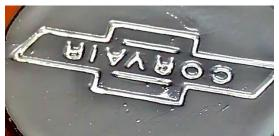
were filled –NOT – then sprayed it several more times. One time I was checking how it would look on the engine, before the paint was hard and I scratched it! Sanded it off and sprayed it for the umpteenth time! Finally decided to quit on this project as it is hardly big enough to see and I'm the only one looking in there anyway! All engine metal is powder-coated satin black.
