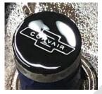
smallest drill bit that I have is 0.013" and that just fit! I carefully ran the slowly turning bit across the grooves Clarence had made and was pleased with how clean it looked. I figured on spraying it with clear Lacquer to fill the grooves.
