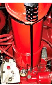
To hold these tall guys down on top of the carbs I had to make looonger "Fran Schmit Spring Loaded J-hooks" - 6 inches long! Turns out I had a nice piece of iron wire that bent when heated and otherwise lent itself to fabrication. With the stacks and the 'Big-X" air cleaner mounted, I can grab the cleaner and shake the car and nothing moves. I think I'm ready to run a test at 6000+RPM and see if they allow the air to turn that corner - smartly! Stay tuned!
