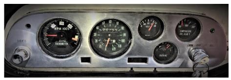
Turns out the guts of the two units would fit inside either can. The Late Model just sits inside a bigger box. BUT, it has a 270° movement so it will give me a nicer swing to the needle, I think. A close-up shows my butchering, next time I will paint better.
