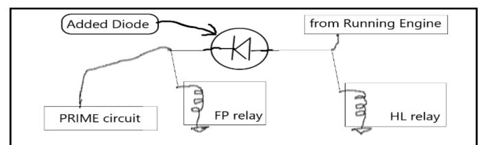
In a CORVAIR with an Elecrtic FP and automatic HL both the FP and the HL come on when the Engine is running. With the added Diode the PRIME will only activate the FP but the Engine control will turn on both the FP and the HL.
