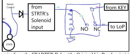
The wire from the STARTER Relay (the Original big Purple wire) is tapped at its original connector, near the Umbilical. Note lack of the Yellow wire. This tap provides the control signal for the Latching Relay.
