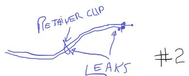
shift cable fit inside of available shrink tubing. The tubing will only shrink to 1/3 of its original size and you want it to shrink down on the shift cable so you can't start out too big. I think I used 1" which would shrink to 3/8". In order to slip the tubing over the anchor (by the O-Ring) I had to cut off the lip of the anchor and make an L-bracket.
