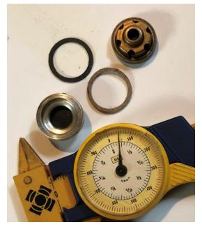
The thing that I didn't expect, was the existence of a teeny little gasket underneath the check valve – where it seats into the housing. This would, I presume, reduce any leakage around the closed valve when it is holding back some pressure. It's only
