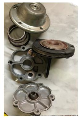
the valve and a spring-loaded flapper lifts off its base to allow the flow through the valve– against its spring. If the pressure changes and the flow attempts to go the other way, the spring pushes the
