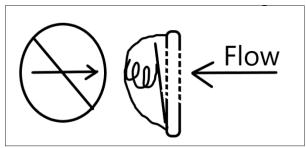
The check valves is what I want to point out today. Here's a sketch of how a check valve looks/works. Fuel is pushed up against
