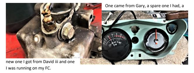
I used the base of a Carb for a heat sink to hold the thermistor and a thermocouple. A "Cyl Head Temp Gauge" (from Clark's) was bolted up tight to that Carb base so they would both be at the same temp, while I read the gauges. First off, I ran a test between the SPYDER dash gauge and the CORSA gauge (by using various resistances to mimic the thermistor's reading — at temp) and got the same readings — so, I would say both gauges read the
