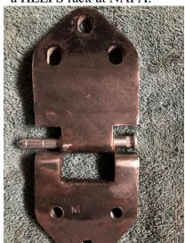
The second pic shows the bushings fitted into the center section.
