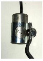
If you are doing this on your bench, at home, you will have to have a wire to bring PLUS to the + terminal of the coil. Half of this setup is bringing + to the coil, so get that part right! The second part of this is a 'manual' Neg terminal connection.
