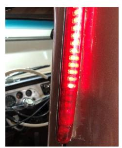
signal, so I put one fixture on each side of the cab. I found these 21 LED units that are both running (TAIL) light and SIGNAL light that mounted up high just like the CHIMSL, but better, I think!
