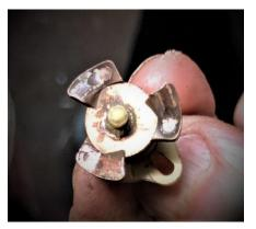
ready for the road, I was curious as to what had gone wrong after 59 years. I had to look inside. The switch has a ratcheting feature which turns a three lobed contact over six terminals. Each time you step on it the three lobed piece rotates just one step. Since four of the terminals (see photo on right) are hot, the rotator puts three of its lobes on two hots and either the high beam bump or the low
