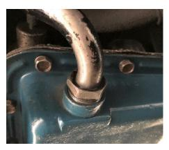
not able to tighten any further. He gave me a one-inch O-ring (with 1/8" wall) that fit exactly inside that port. I tilted my '64 up high, with a jack, (and jack-stands!) so the oil would flow to the other side and opened up the connection. I put in the '1-incher', before a cup of oil could escape. Bingo! No Drip.
