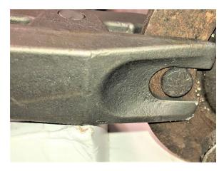
Here we see two fingers behind the flange. The force applied by the Ball-joint tool's screw will bring these two towards the single finger.
