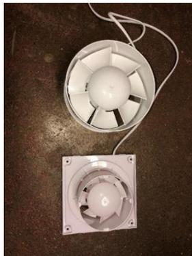
Put two T/Cs in the two pipes on my FC and found the average temp to be about 150°F. So, mixing that four times (about) should get me down to around 100°F air - that would hit the plastic blades of the fan. OK, I think.
