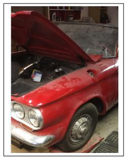
**1963** Corvair Monza convertible; body and suspension restored; engine is not assembled. Aftermarket seats, fuel injection (still in box), many other new parts.
