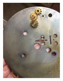
On the left you see the little guys that accomplish that 'turn around'. The long shaft, from the front, drives the top gear in the photo. Obviously turning all the others and carrying the 'turning' towards the center hole. The clock mechanism used to drive the hands through the center hole in this plate.
