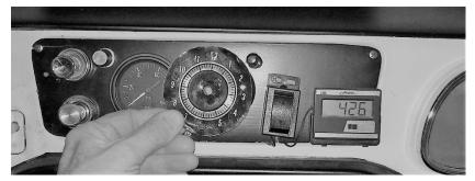
mine as well; however, someone before me had hacked a huge hole in that spot for a Tachometer. I, in turn, needed a place for some instruments when I switched to a Spyder dash. All mounted together on a panel shaped to fit the indent of the FC dash.
