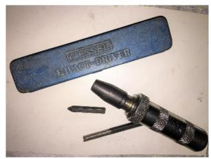
brass boys from way down in the hole. An IMPACT driver, that I have, uses a 5/16" hex drive. So I
