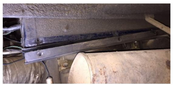
On one side I was missing the big washer between #5 and 6 so I asked Clark's for one. They said sorry – don't have them. This washer is shaped to hold #6 in proper position, so I had to make a shaped washer out of heavy stock. It
