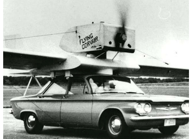
October 26 1970 in Orange, Massachusetts: Erwin Stockwell, 62, who has flown for 37 years, "pilots" his aeromobile, a standard car with wings, propeller and an extra engine added, down the runway of Municipal Airport on a trial run. Stockwell, retired precision tool maker, assembled his vehicle behind his home with federal Aviation Administration approval. He hopes to have his invention ready for flight this spring.
