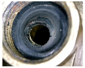
have solved the problem of availability of 9mm O-rings and may have come up with an even better gasket material. The commercial O-rings I have used were often broken (splintered) after the fitting had been tightened. They didn't leak but were not fit to be put back in service. At '4 for a buck' they were affordable but the pieces did land in the in-carb filter and looked scary in there.
