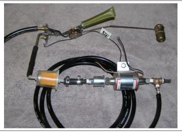
The photo on the left shows how all the parts used to construct this new format fit together. The return line's Tee fitting has the eight foot hose attached at both ends. The repaired float is shown ready for service.
